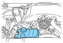
If the engine coolant has not been checked at the recommended interval, the engine coolant reservoir may become empty. If this occurs, add engine coolant to the reservoir. For more information on engine coolant maintenance, refer to *Adding engine coolant* in this chapter.
